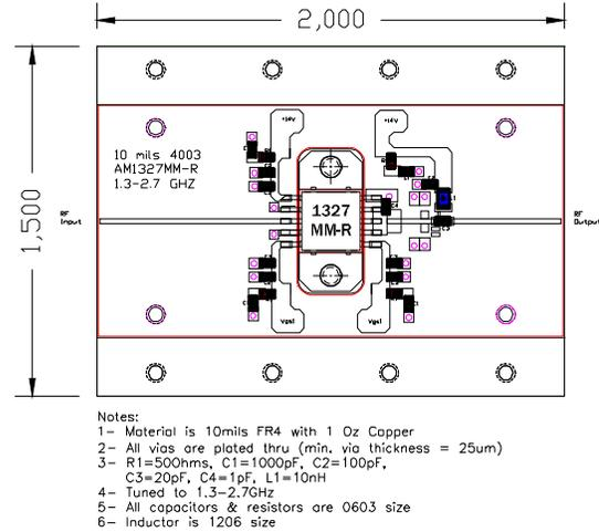
Figure 3: Off-chip output matching circuit on PCB (10-mil thick, FR4 PCB)
