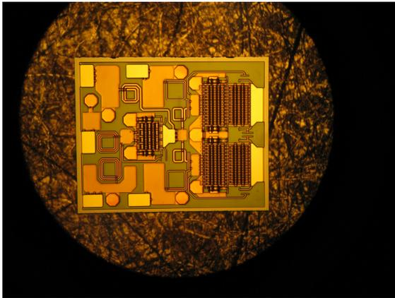
Figure 2a. Photo of a 2-stage, 2HIFET MMIC PA.
