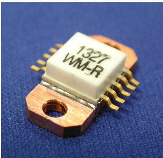
Figure 2b. MMIC in a ceramic package with a copper flange.
