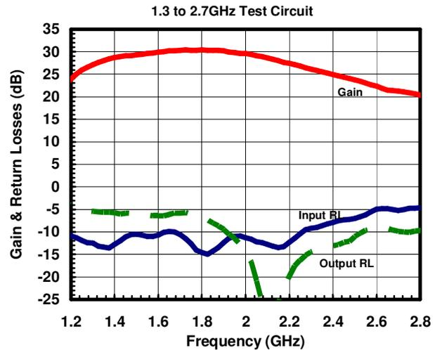
Figure 4. Measured small signal gain versus frequency.
