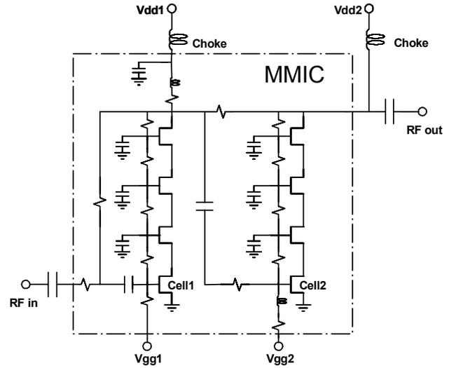
Fig.2. MMIC circuit schematic diagram.
