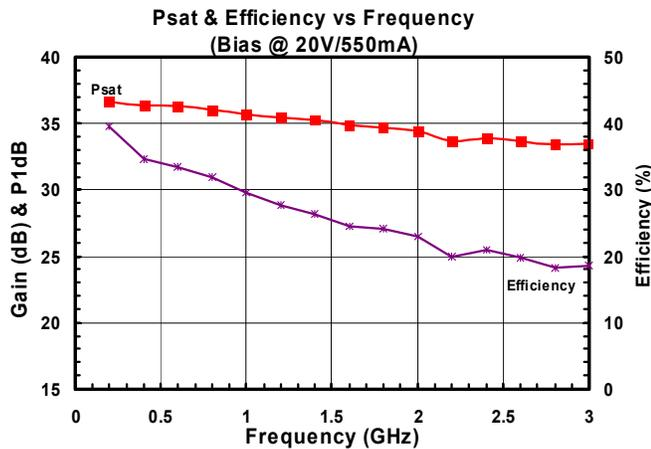
Fig. 8. Saturated power & efficiency versus frequency.
