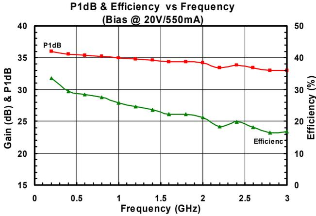
Fig. 7.  $P_{1dB}$  & efficiency versus frequency.
