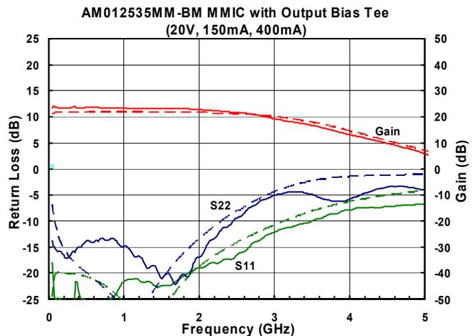
Fig. 6. Small signal measurements & simulation (dashed).
