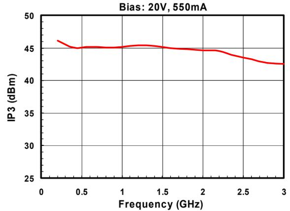
Fig. 9. IP3 versus frequency.
